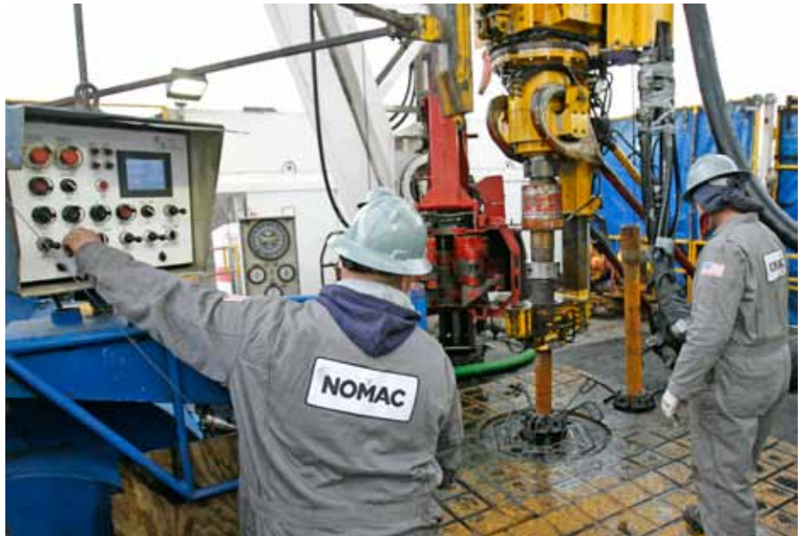
Workers prepare to change drilling pipes on the rotary table of a natural gas drilling rig in the United States. REUTERS/Tim Shaffer
